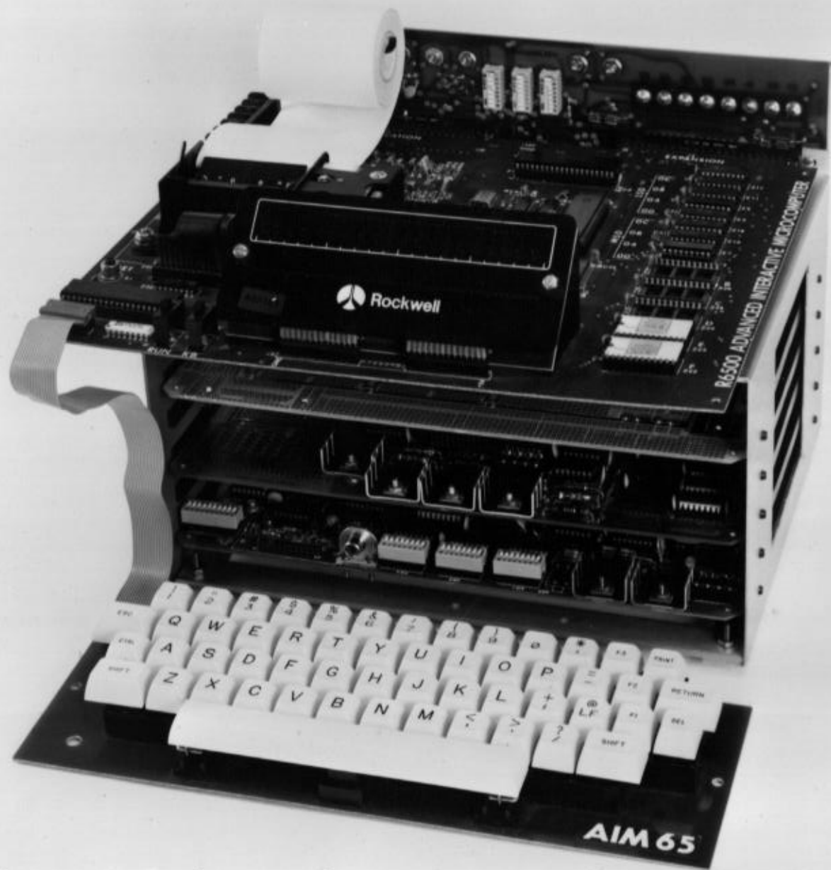
MOTHER BOARD HOLDING EXPANSION BOARDS FOR AIM65
